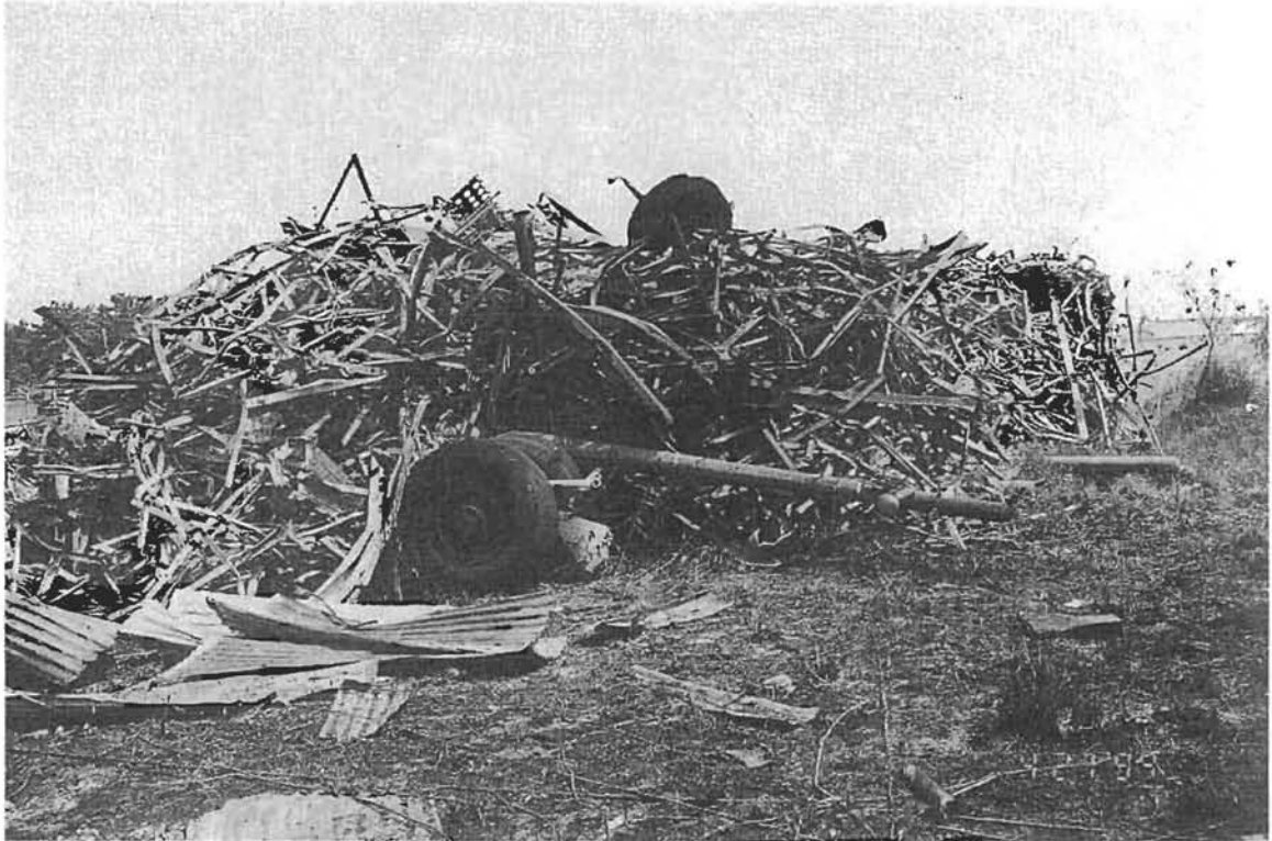
Photo.24 Tires of the Right Main Landing Gear
