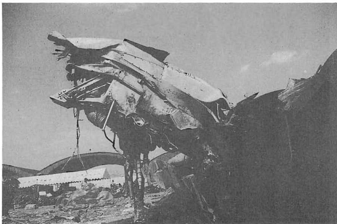
Photo.34 No.2 Engine Pylon
