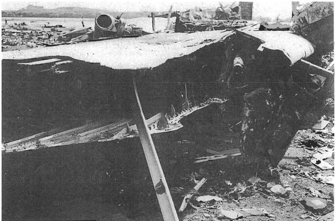
Photo.20 Fractures of the Right Wing
