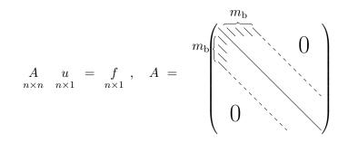
Figure 27.1: A banded matrix with bandwidth  $m_{\rm b}$ .
