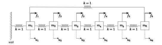
Figure 27.5: "Cyclic" spring-mass system with n = 6 masses.
