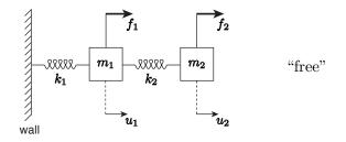
Figure 25.1: A system of two masses and two springs anchored to a wall and subject to applied forces.
