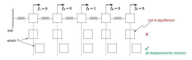
Figure 27.8: Response of a n = 5 spring-mass system to unit loading on mass 3.
