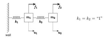
Figure 26.1: n = 2 spring-mass system.
