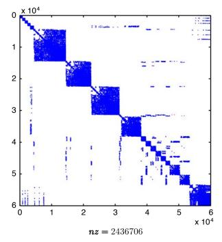
Courtesy of Dr. Phuong Huynh. Used with permission. Figure 24.2: Structure of stiffness matrix K.
