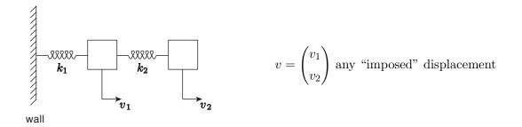
Figure 25.4: Spring-mass system: imposed displacements v.
