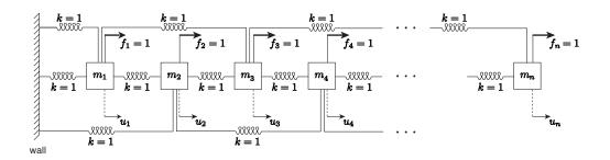
Figure 27.2: A spring-mass system whose equilibrium state calculation gives rise to a pentadiagonal matrix.
