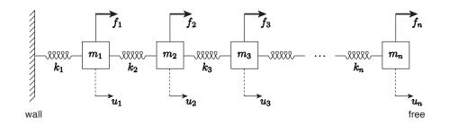
Figure 25.13: System of n springs and masses.
