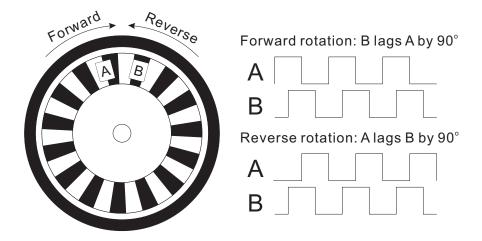
Figure 1.3: A quadrature rotary encoder and its output for clockwise and counterclockwise rotation.
