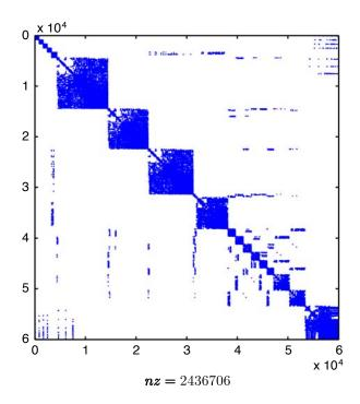
Figure 24.2: Structure of stiffness matrix K.
