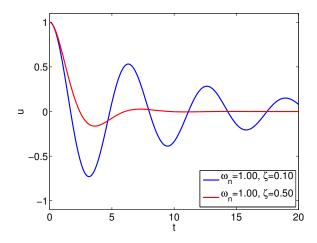
Figure 21.17: Response of underdamped spring-mass-damper systems.
