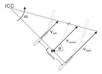
Figure 1.4: Robot trajectory.
