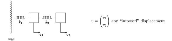
Figure 25.4: Spring-mass system: imposed displacements v.
