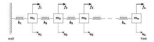
Figure 25.13: System of n springs and masses.
