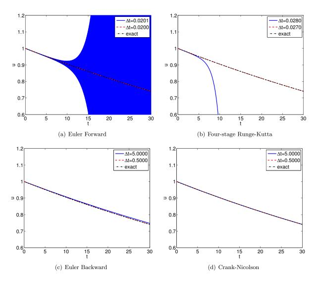
Figure 21.21: Comparison of numerical integration schemes for an overdamped spring-mass-damper system with  $\omega_n = 1.0$  and  $\zeta = 50$ . Note that the time step used for the explicit schemes are different from those for the implicit schemes.
