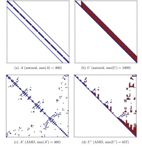
Figure 27.7: Comparison of the sparsity pattern and Gaussian elimination fill-ins for a n=100 "outrigger" system resulting from natural ordering and an equivalent system using the approximate minimum degree (AMD) ordering.
