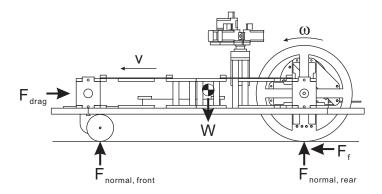
Figure 15.1: A mobile robot in motion.
