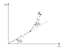
Figure 29.2: Schematic of robot arm.
