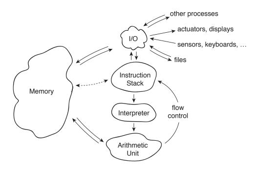
Figure 4.1: Virtual Processor
