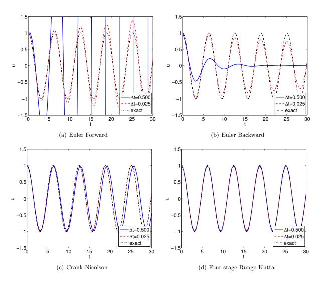
Figure 21.20: Comparison of numerical integration schemes for an undamped spring-mass system with  $\omega_n=1.0$ .
