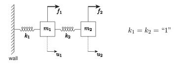
Figure 26.1: n = 2 spring-mass system.
