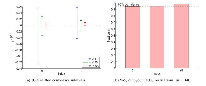
Figure 19.5: a) The variation in the 95% confidence interval with the sampling size m for the linear model fitting. b) The frequency of the individual confidence intervals  $I_0$  and  $I_1$  including the true parameters  $\beta_0^{\text{true}}$  and  $\beta_1^{\text{true}}$  (0 and 1, respectively), and  $I_0^{\text{joint}} \times I_1^{\text{joint}}$  jointly including ( $\beta_0^{\text{true}}, \beta_1^{\text{true}}$ ) (all).
