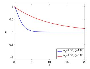
Figure 21.18: Response of overdamped spring-mass-damper systems.
