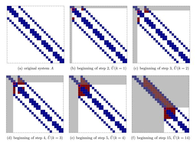
Figure 27.3: Illustration of Gaussian elimination applied to a  $25 \times 25$  "outrigger" system. The blue entries are the entries present in the original system, and the red entries are "fill-in" introduced in the factorization process. The pivot for each step is marked by a red square.
