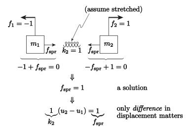
Figure 25.11: Scenario II. (Note on the left mass the  $f_1$  arrow indicates the direction of the force  $f_1 = -1$ , not the direction of positive force.)
