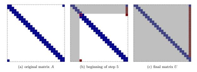
Figure 27.6: Illustration of Gaussian elimination applied to a  $25 \times 25$  "arrow" system. The red entries are "fill-in" introduced in the factorization process. The pivot for each step is marked by a red square.
