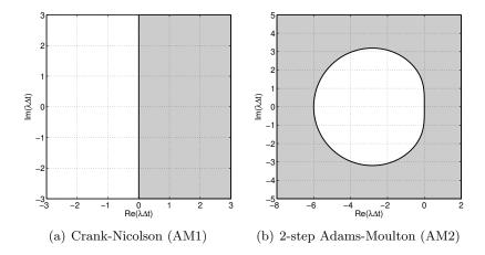
Figure 21.12: The stability diagrams for 2-step Adams-Moulton methods.
