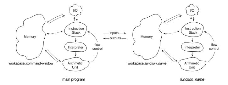
Figure 6.1: Two Virtual Processors
