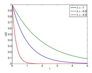
Figure 21.1: Solutions to the homogeneous equation.
