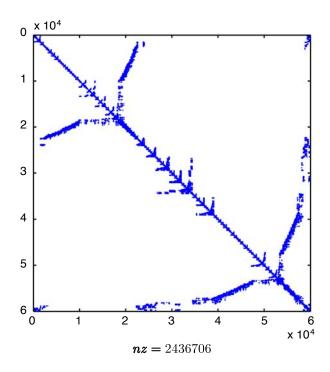
Figure 24.3: Structure of reordered stiffness matrix K'.
