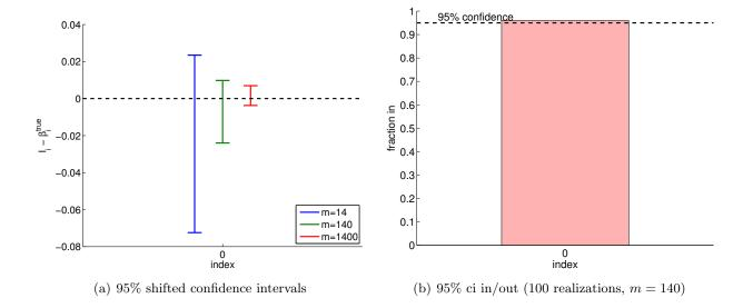
Figure 19.3: (a) The variation in the 95% confidence interval with the sampling size m for the constant model fitting. (b) The frequency of the confidence interval  $I_0$  including the true parameter  $\beta_0^{\text{true}}$ .
