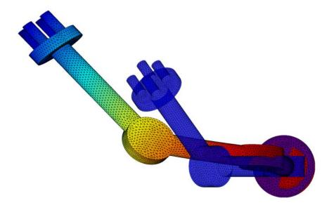
Figure 24.1: Deflection of robot arm.
