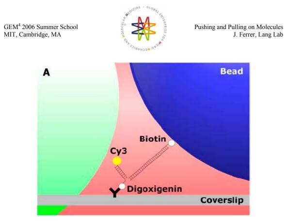
FIGURE 2. Unzipping geometry for a 15-bp dsDNAsystem. It is attached on one end to a trapped bead via a biotin–streptavidin interaction and immobilized on the other end by means of a digoxigenin-antibody linkage. The 15-bp region of interest is labeled with a Cy3 fluorophore to confirm the location and timing of the unzipping mechanical event.
