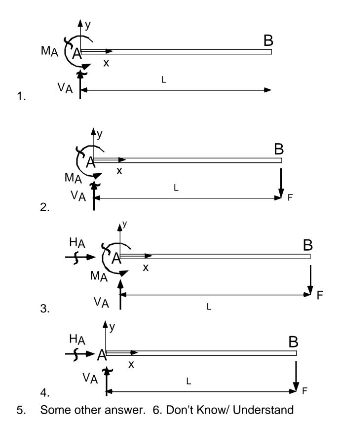
M4CQ2 For which of the beams shown below can one solve for the reaction forces with the information given?
