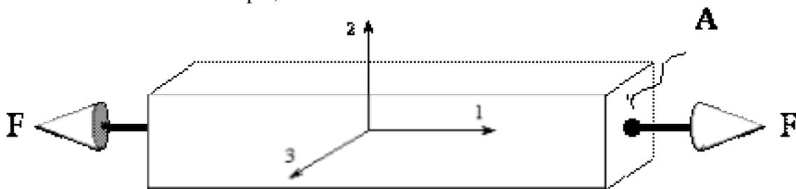
Figure 1. Material Under an Axial Load
