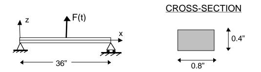
(a) Determine the natural frequencies and the mode shapes for the first three modes.
