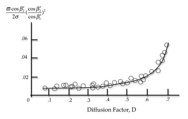
Image by Manuel Martinez-Sanchez. Adapted from Fig. 5.12 in Kerrebrock, Jack L. *Aircraft Engines and Gas Turbines*. 2nd edition. MIT Press, 1992.
