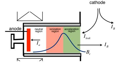
As will be discussed later, one of the factors determining the overall efficiency  $\eta$  of the device is the anode efficiency,
