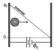
Ignoring space charge effects, we have a constant electric field pushing the ion to the right. Through a simple energy balance, we find an expression for the velocity of ions arriving at the second electrode. If such electrode were transparent to ions, we would then have a thruster with specific impulse,
