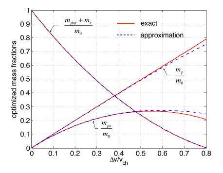
Figure 2: Optimized mass fractions as a function of  $\Delta v/v_{ch}$
