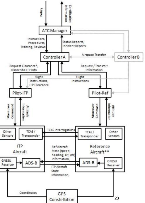
Image: Public Domain. Figure 7: Safety Control Structure for ATSA-ITP. Fleming, Cody Harrison, Melissa Spencer, Nancy Leveson et al. "Safety Assurance in NextGen." March 2012. NASA/CR-2012-217553.
