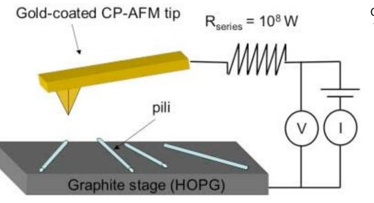
Schematic of the electronic connection of the AFM tip in a conducting probe atomic force microscope (CP-AFM). HOPG, highly oriented pyrolytic graphite. Correspondence between pilus current and applied voltage demonstrating the linear, ohmic, response characteristic of a true conductor.
