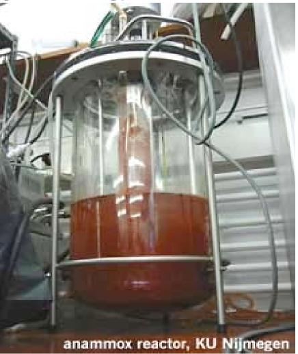
Anammox means "anaerobic ammonium oxidation". Anammox is both a new low-cost method of N-removal in wastewater treatment, and a spectacular microbial way of life - **woo - woo !** Courtesy of the Department of Microbiology at Radboud University Nijmegen. Used with permission. Broda E: Two kinds of lithotrophs missing in nature. Z Allg Mikrobiol 1977, 17:491-493.
