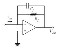
Figure 3: Transimpedance amplifier circuit.
