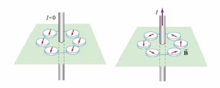
Figure 9.3.1 Deflection of compass needles near a current-carrying wire
