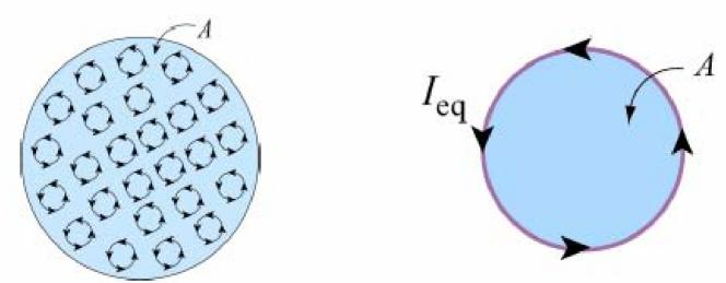
Figure 9.6.2 (a) Top view of the cylinder containing magnetic dipole moments. (b) The equivalent current.
