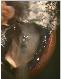
5.4 One electrode placement. The arrow is aligned aling the electrode entering from the right. The electrode tip is in the saline and just about to contact the tissue. It is at this point that you should turn on your amplifier, etc.
