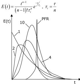
**Figure 15.** E(t) plots for 1, 2, 4, and 10 tanks and a PFR. Notice how the E(t) curve approaches the PFR pulse as more tanks are used.
