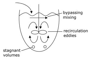
**Figure 3.** A real mixed tank. In a real mixed tank there are portions that are not well mixed due to stagnant volumes, recirculation eddies, and mixing bypasses.
