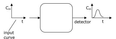
**Figure 6.** Schematic of a residence-time distribution experiment. The input curve enters the reactor; a detector detects concentration changes in the output stream.
