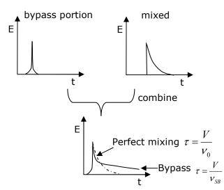
Figure 10. Residence-time distribution determination for a bypass.
