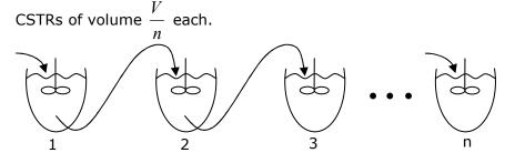
**Figure 14.** n tanks in series. The output of tank 1 is the input to tank 2. The output is sampled at tank n for dispersion.
