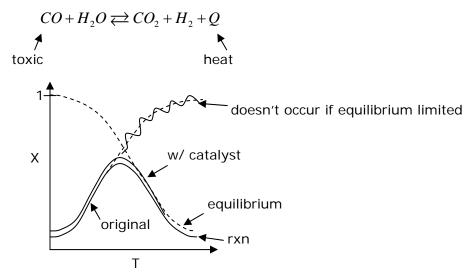
Figure 3. Conversion (X) versus Temperature (T).
