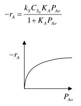
**Figure 3.** Reaction rate vs. initial partial pressure of A for the surface reaction limiting case.
