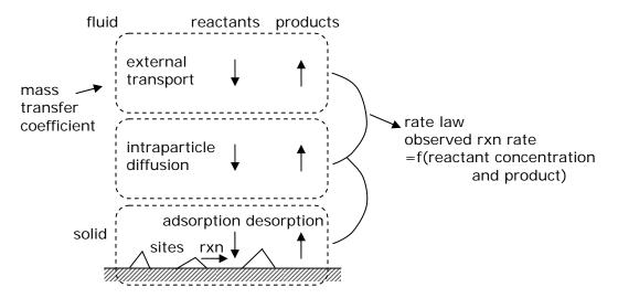
Figure 1. Schematic of surface reaction kinetics.
