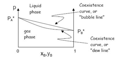
This allows us to see the compositions of both liquid and gas phases
