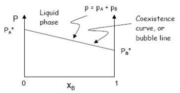
The gas phase is described by  $y_A$  or  $y_B$ . If T and  $x_A$  are given, then  $y_A$  and  $y_B$  are fixed (by Gibbs phase rule). That is, if T and the composition of the liquid phase are known, then the composition of the gas phase is determined.
