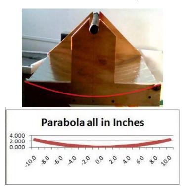
Figure 1: This graphic shows flattened parabolic shape of Focus. The actually focus is 10 inches above the vertex. In the actual model, the focus is at the center of the copper pipe.
