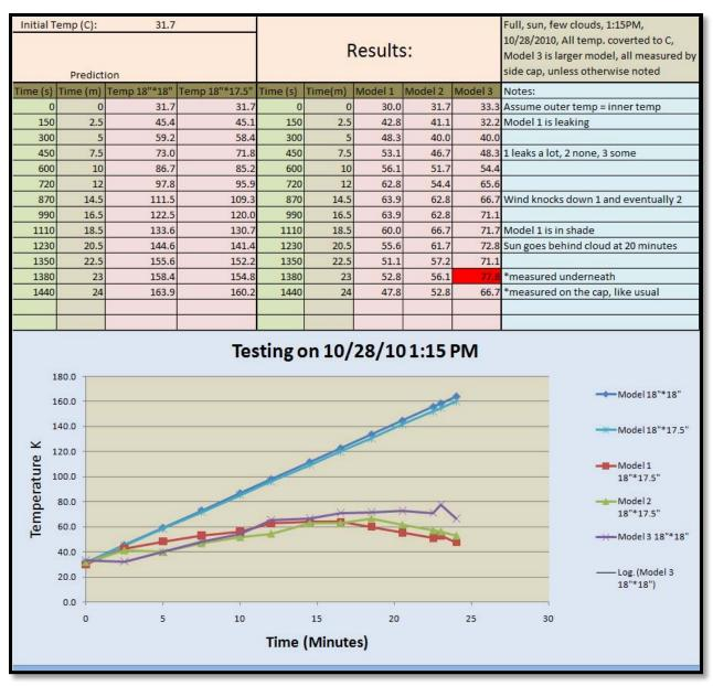
Table 3 and Figure 8: The data from one afternoon test using three models. Models 1, 2, and 3 are actual models constructed. The first two "models" are the linear thermal models. The highlighted value is the maximum temperature registered among the three models.
