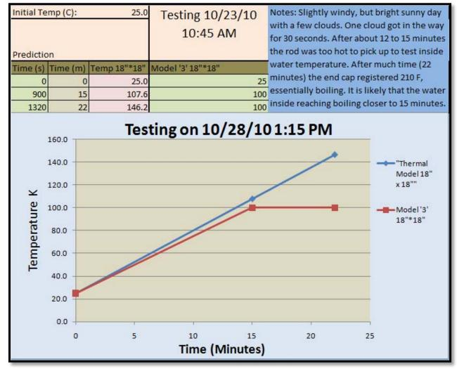
Table 2 and Figure 7: This initial tested showed that on prime conditions (bright sun), focus can reach boiling. This design was the 18" by 18" model. It has two data points for boiling because the water had likely reached boiling by about 12 to 15 minutes, but it was not formally measured until 22 minutes
