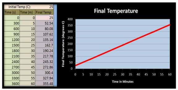
The water should hit boiling in a little less than 14 minutes given that the water starts at 25 °C.
