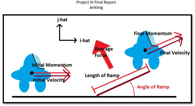
Figure 17: This is a simple sketch on which the model is based. Note the time to clear the ramp is simply the length of the ramp divided by the initial speed.
