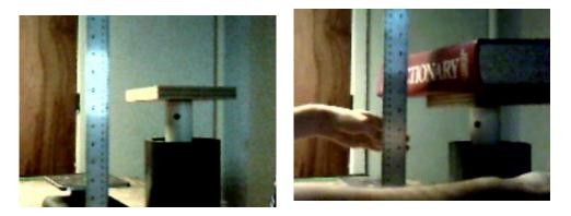
Figures 13-14: These are two pictures of the testing setup for the dashpot. Weights (books) were added to the dashpot and the rate of compression was measured using a video recorder on a laptop. The ruler measured the distance dropped and the video footage measured the time elapsed. The terminal velocity of the dashpot was measured in this way. Shown in the left picture is the scale that was used to measure the weight of the books.
