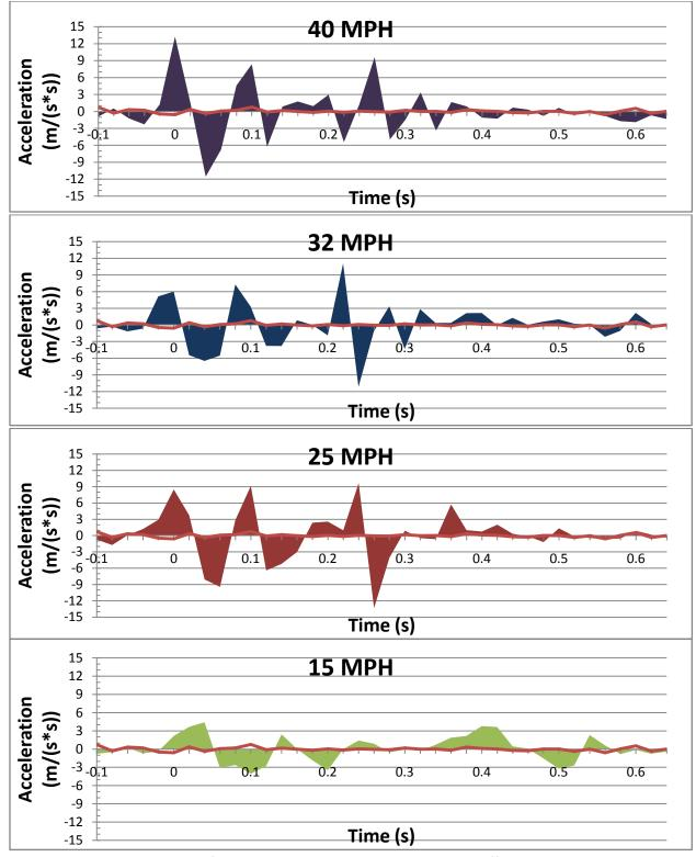
Figure 8-12: The acceleration from a speed table or speed bumps at different speeds. The red line is normal vibrations of the car without a speed bump. Notice the differences in magnitude of the accelerations and their duration.
