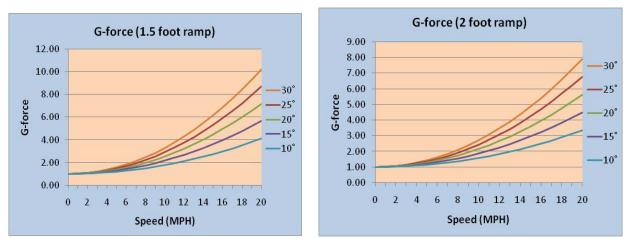
Figures 18 and 19: Graphs of the average g-forces applied to a vehicle riding over 1.5 and 2 foot angled ramps. Notice the changes in scale that reflect change in the magnitude of the average acceleration.
