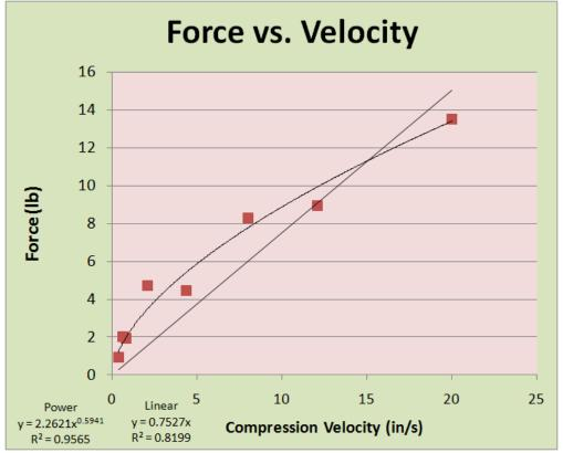
Figure 15: A graph showing the relationship between the compression velocity and the resistive force. It is important to note that for testing, compression velocity was a dependent variable of the force applied, but the inverse that force is dependent upon compression velocity is more applicable to Jerkling.
