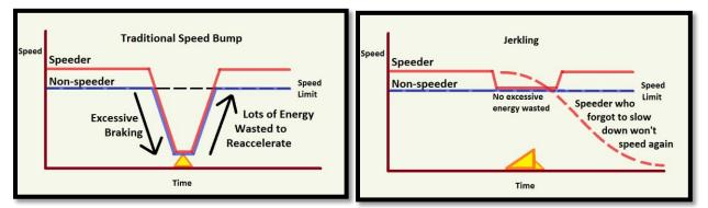
Figures 1 and 2: The left figure is a graph that depicts the speed of two vehicles traveling over a traditional speed bump. The right figure is a graph that depicts the speed of two vehicles traveling over Jerkling.
