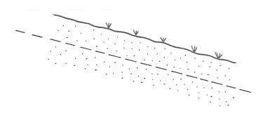
Figure 10-3. The force of gravity on a layer of deformable material on a slope.
