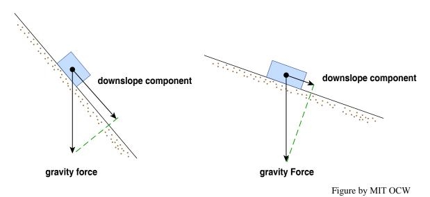
Figure 10-1. Resolving the force of gravity into a component in the downslope direction. The lengths of the arrows represent the magnitudes of the components of the gravity force. Left: a steep slope. Right: a gentle slope.
