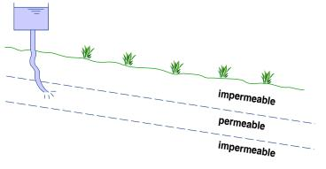
Figure by MIT OCW Figure 10-6. Increase in pore pressure in a subsurface layer.
