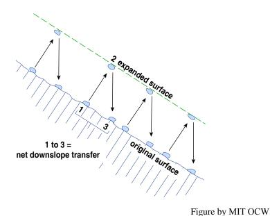
Figure 10-7. Sawtooth path of a surface particle caused by expansion and contraction of the soil. (From Bloom, 1998)
