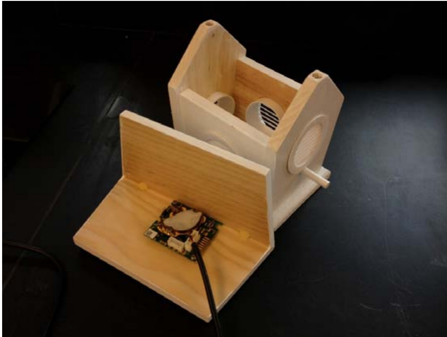
Portable CO 2 meter/data logger in a bird house
