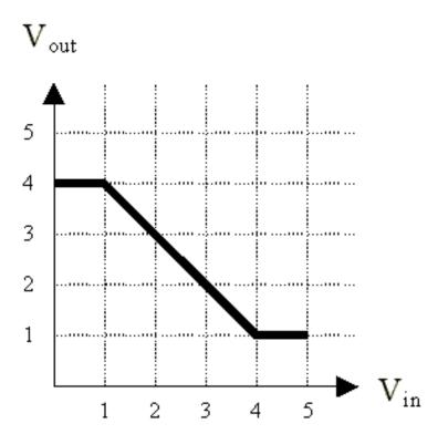
Can this device be used as a combinational device in a logic family with 0.75V noise margins?
