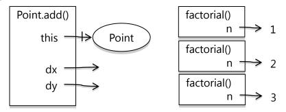
The left example shows Java's *this* reference, which refers to the object on which the method was called. The right example shows that stacks are drawn upwards: when a method calls another method, the new stack frame is drawn on top. This factorial function recursively calls itself with steadily decreasing values for the parameter *n*.
