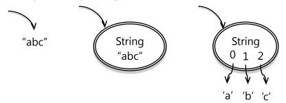
Finally, when we're talking about the concrete internal representation of a string in Java, we might draw a picture like this, which shows the string's character array:
