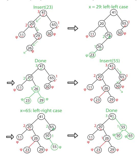
Figure 7: Illustration of AVL Tree Insert Process
