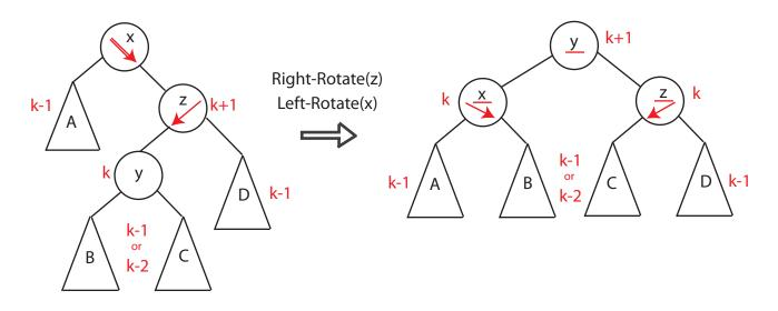
Figure 6: AVL Insert Balancing
