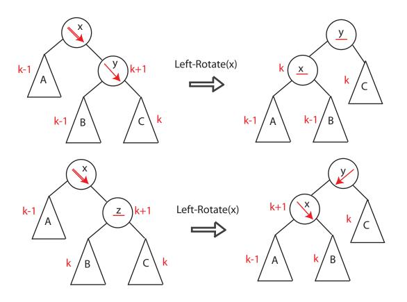
Figure 5: AVL Insert Balancing
