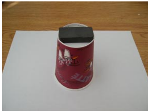
Figure 5: Place the cup upside down. Squeeze the magnet between the ledge. This should hold the magnet firmly in place.
