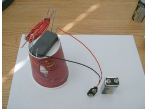
Figure 9: Hang your coil on the paper clips. Make sure your coil is sitting centered above the magnet. Attach the battery strap to the paper clips and you are done!
