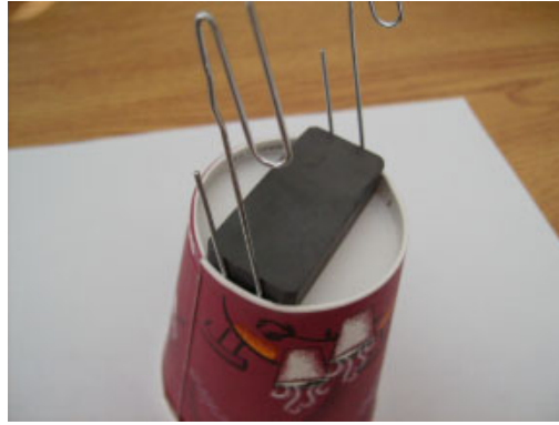
Figure 7: Insert the paper clips between the ledge and the side of the magnet as shown in the figure.
