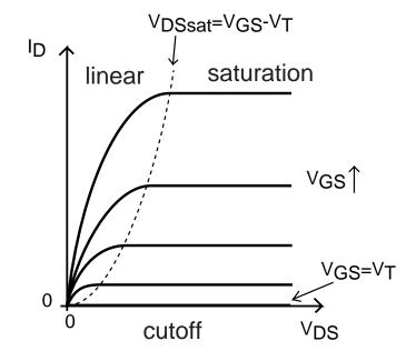
$$I_{Dsat} = \frac{W}{2L} \mu_n C_{ox} (V_{GS} - V_T)^2$$
