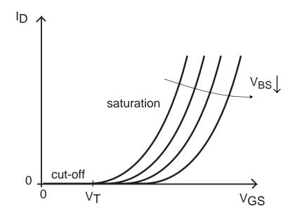
Backate characteristics ( $V_{BS} = 0, -1, -2, -3 V, V_{DS} = 3 V$ ):
