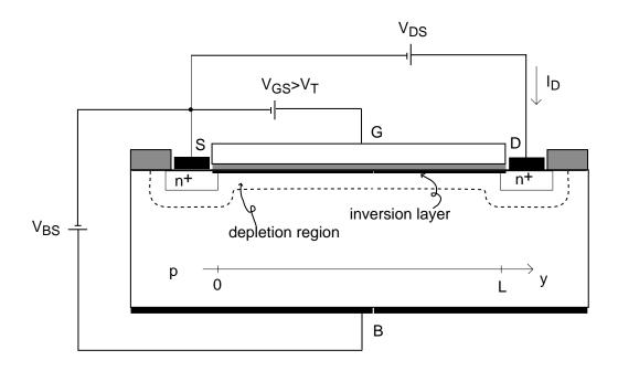
Body contact allows application of bias to body with respect to inversion layer,  $V_{BS}$ .
