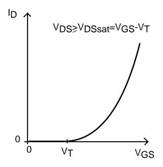
$\Box$  What happens when  $V_{DS} = V_{GS} - V_T$ ?
