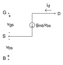
Complete MOSFET small-signal equivalent circuit model for low frequency:
