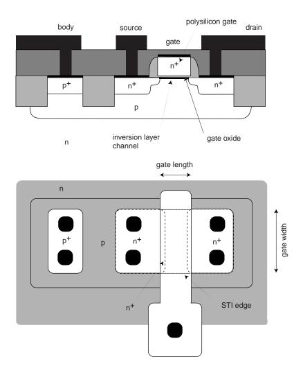
Body-to-source capacitance = source junction capacitance:
