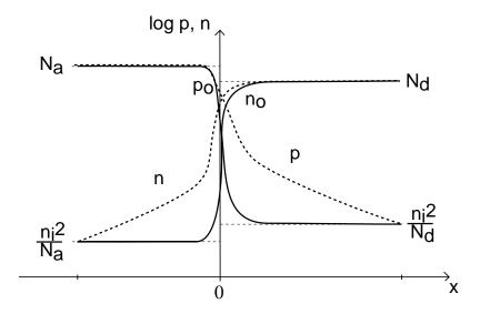
• Reverse bias: minority carriers extracted by SCR  $\Rightarrow$  generated at surface and diffuse through QNR
