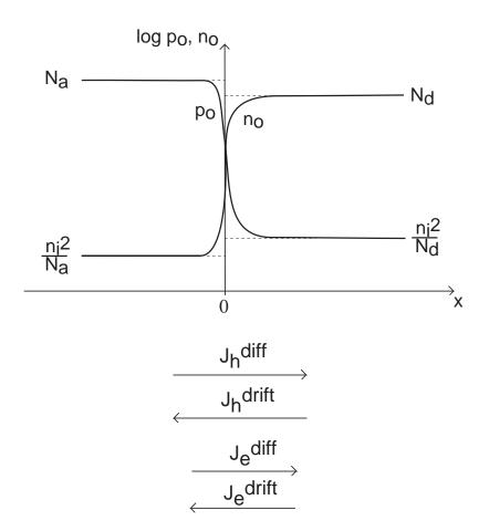
Inside SCR in thermal equilibrium: dynamic balance between drift and diffusion for electrons and holes.
