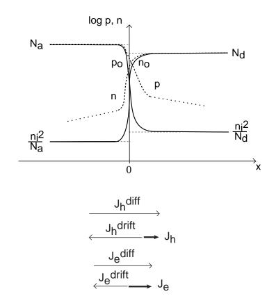
Current balance in SCR broken:
