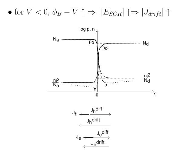
Current balance in SCR broken:
