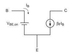
• Saturation: device flooded with minority carriers. Not useful. For bias calculations:
