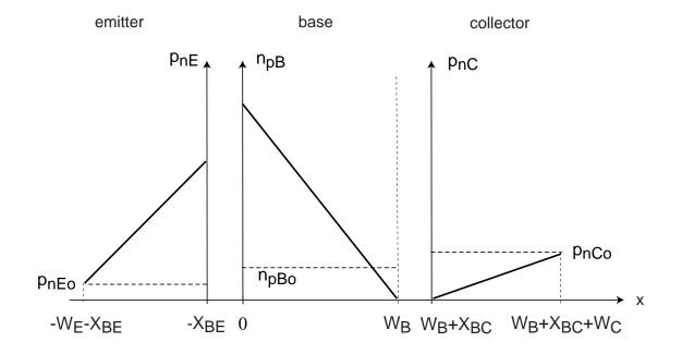
• Emitter injects electrons into base, collector collects electrons from base:
