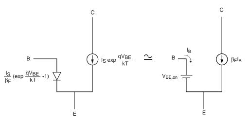
For today's technology:  $V_{BE,on} \simeq 0.7 V$ .  $I_B$  depends on outside circuit.
