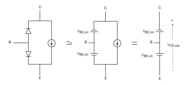
Today's technology:  $V_{CE,sat} = V_{BE,on} - V_{BC,on} \simeq 0.2 V$ .  $I_B$  and  $I_C$  depend on outside circuit.
