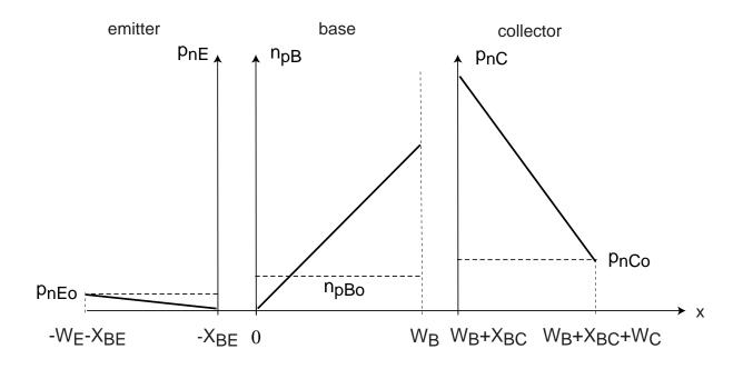
• Collector injects electrons into base, emitter collects electrons from base:
