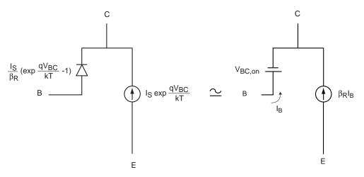
For today's technology:  $V_{BC,on} \simeq 0.5 V$ .  $I_B$  also depends on outside circuit.
