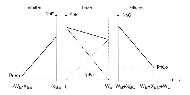
Saturation is superposition of forward active + reverse:
