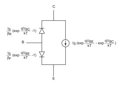
Three parameters in this model:  $I_S$ ,  $\beta_F$ , and  $\beta_R$ . Model equivalent to Ebers-Moll model in text. Simplifications of equivalent-circuit model:
