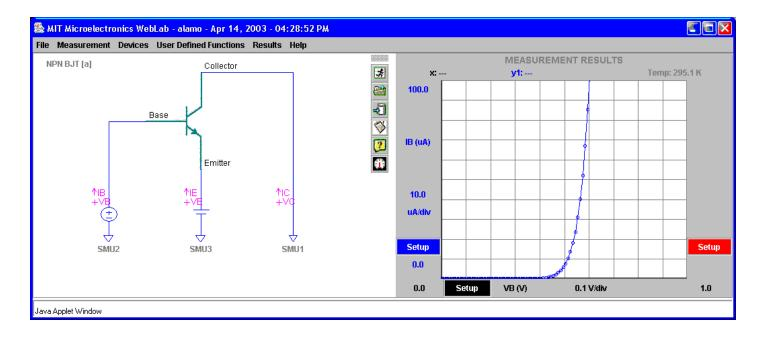
• Saturation:  $V_{BE} > 0, V_{BC} > 0$
