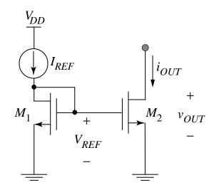
$$I_{OUT} \simeq \frac{1}{2} \left(\frac{W}{L}\right)_2 \mu C_{ox} (V_{REF} - V_T)^2$$
