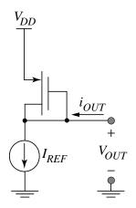
Same operation and characteristics as NMOS voltage source. PMOS needs to be bigger to attain same  $R_{out}$ .
