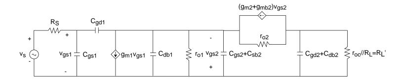
Time constants associated with  $C_{gs1}$  and  $C_{gd2} + C_{db2}$  have not changed.
