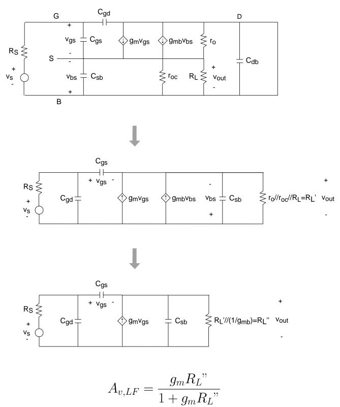
$C_{sb}$  shows up at same location as  $C_{db}$  before, then bandwidth is:
