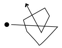
Characteristic time constant of thermal motion - mean free time between collisions:
