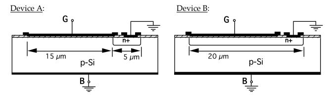
Both of these devices are made on p-type silicon with a net doping level of  $10^{17}$  cm<sup>-3</sup>, and are 20  $\mu$ m wide normal to the page. The n<sup>+</sup> regions are doped to  $10^{18}$  cm<sup>-3</sup>, and the n<sup>+</sup>-p junction is 1  $\mu$ m from the top surface. The thin oxide is a high quality
