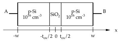
Use the depletion approximation model when solving this problem. Assume that the depletion region widths are less than w/2. The drawing may not be to scale.
