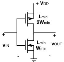
This minimum size inverter is shown above. The gate delay,  $\tau_{GD}$ , of this minimum size inverter is found to be 100 ps (10<sup>-10</sup> s) when the fan-out is one. We will call this gate delay the minimum gate delay,  $\tau_{min}$ .
