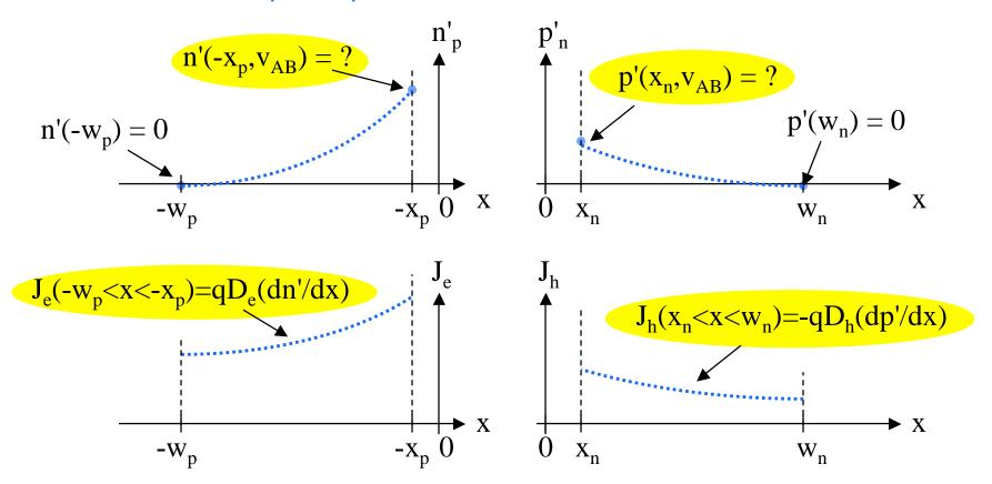
Having  $J_e(x)$  for  $-w_p < x < -x_p$ , and  $J_h(x)$  for  $x_n < x < w_n$ , we can get  $i_D$ because we will argue that  $i_D(v_{AB}) = A[J_e(-x_p, v_{AB})+J_h(x_n, v_{AB})]...$ ...but first we need to know n'( $-x_p, v_{AB}$ ) and p'( $x_n, v_{AB}$ ). Clif Fonstad, 9/29/09 We will do this now.
