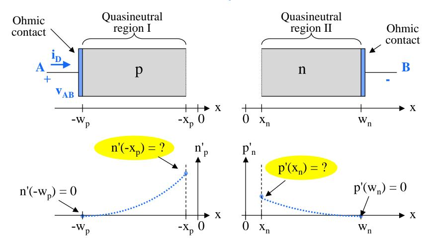
If we knew n'(- $x_p$ ) and p'( $x_n$ ), we could solve the flow problems and we could get n'(x) for - $w_p$ <x<- $x_p$ , and p'(x) for  $x_n$ <x< $w_n$ ... Clif Fonstad, 9/29/09 ....and knowing n'(x) for  $-w_p < x < -x_p$ , and p'(x) for  $x_n < x < w_n$ , we can find  $J_e(x)$  for  $-w_p < x < -x_p$ , and  $J_h(x)$  for  $x_n < x < w_n$ .
