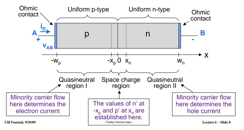
**The p-n Junction Diode:** the game plan for getting  $i_D(v_{AB})$ We have two QNR's and a flow problem in each:
