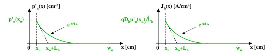
**Case II - Short base:**  $w_n \ll L_n$  (the situation in most Si diodes and transistors)
