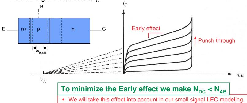
Punch through - base width modulation taken to the limit When the depletion region at the B-C junction extends all the way through the base to the emitter, I<sub>C</sub> increases uncontrolably. Punch through has a similar effect on the characteristics to that of Clif Fonstad, 10/6/09 reverse breakdown of the B-C junction.
