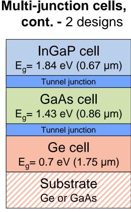
A 3 -junction design (3 lattice-matched cells connected in series by tunnel diodes)
