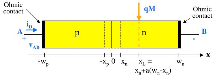
What is  $i_D(v_{AB}, M)$ ? Use superposition to find the answer:  $i_D(v_{AB}, M) = i_D(v_{AB}, 0) + i_D(0, M)$
