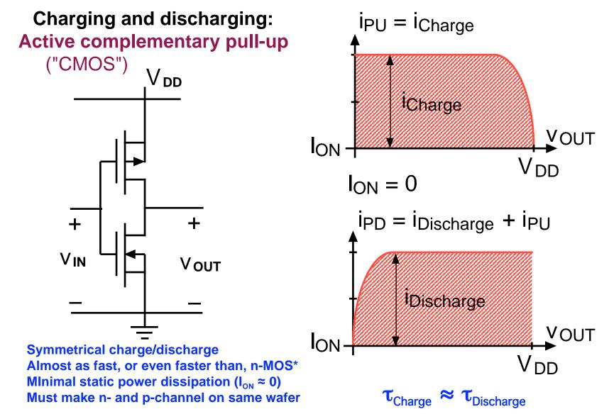
Clif Fonstad, 10/29/09 \* The input capacitance is 3x larger, but the interconnect capacitance Lecture 14 - Slide 21 is the same, so it depends on which of the two is dominant.
