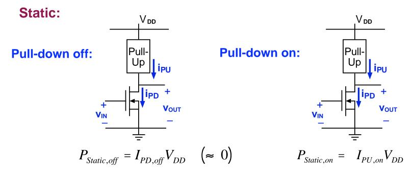
To estimate the total static power we assume the typical pull-down is off half the time and on half the time.
