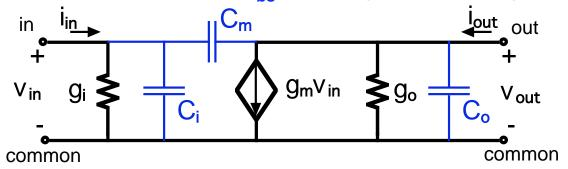
Most linear circuits are designed to operate at frequencies where the capacitors look like open circuits. We can thus do our designs neglecting them.\*
