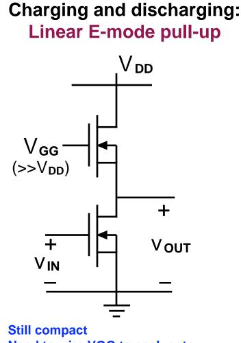
Need to wire VGG to each gate Need second supply Not faster than linear resistor
