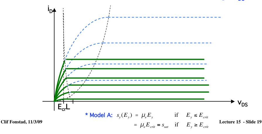
If the channel length, L, is sufficiently small we can simplify the model even further because the carrier velocity will saturate at such a small  $v_{DS}$  that for  $v_{DS} \ge E_{crit}L$  the inversion layer will be uniform and all the carriers will be drifting at their saturation velocity. In this situation (the saturation region) we will have:
