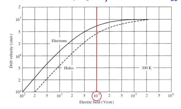
Clearly the velocity of the electrons and holes in the channel will be saturated at even low values of v<sub>DS</sub>!
