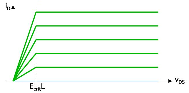
Note first that in the forward active region where  $v_{DS} \ge E_{crit}L$ , the curves in the output family are evenly spaced, indicating a constant  $g_m$ :  $g_m \equiv \partial i_D / \partial v_{GS} \Big|_O = W s_{sat} C_{ox}^*$
