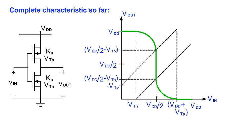
**NOTE:** We design CMOS inverters to have  $K_n = K_p$  and  $V_{Tn} = -V_{Tp}$  to obtain the optimum symmetrical characteristic.
