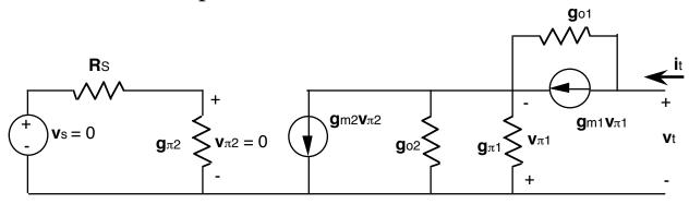
We see immediately that  $i_t = -(g_{02} + g_{\pi 1}) v_{\pi}$ , and at the one node in the circuit we can write
