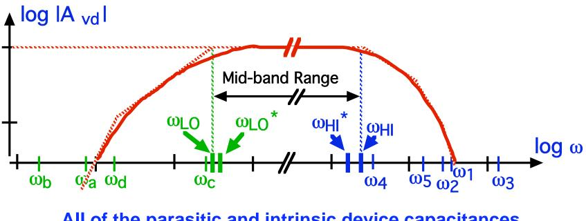
All of the <u>parasitic and intrinsic device capacitances</u> are effectively open circuits
