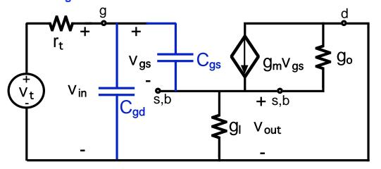
C<sub>gs</sub> is in the Miller position, but the voltage gain is one so there is no Miller effect.
