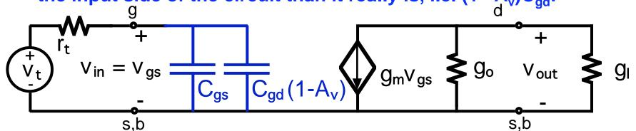
This "magnification" of a capacitor bridging the input and the output of a voltage amplifier, as  $C_{gd}$  does here, by  $|A_v|$  is called the <u>Miller effect</u>.
