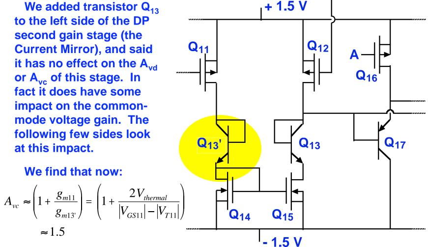
Remember that it is possible to make the bias currents in the two legs of the mirror  $(Q_{11}/Q_{14})$  and  $Q_{12}/Q_{15}$ ) different by making the transistors widths different. Clif Fonstad, 12/3/09 Lecture 23 - Slide 2
