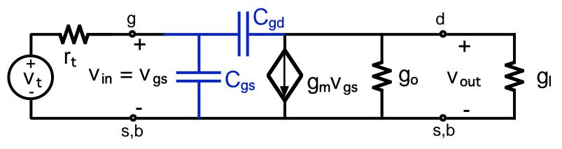
The resistance,  $R_{gs}$ , seen by  $C_{gs}$  with  $C_{gd}$  removed is  $1/g_t$ , so
