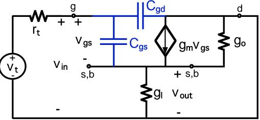
**Repositioning**  $C_{qd}$  makes the situation clearer:
