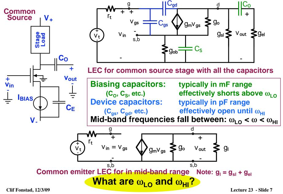
**Estimating** ω<sub>HI</sub> - Open Circuit Time Constants Method
