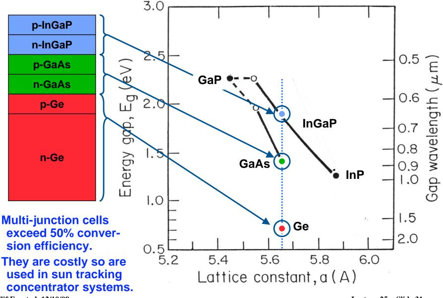
**Solar Cells:** Multi-junction solar cells InGaP/GaAs/Ge
