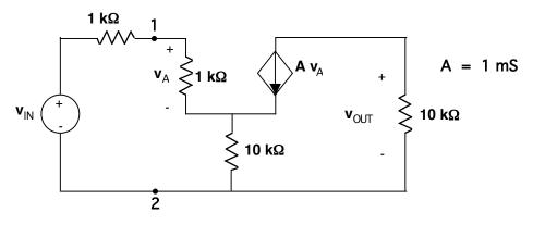
(a) What is the voltage  $v_{OUT}$  when the input voltage,  $v_{IN}$ , is 2 Volts?
