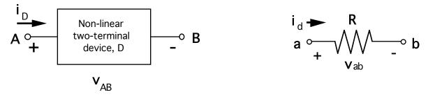
A linear equivalent circuit for the device D valid for small signal operation about a bias point,  $v_{AB} = V_{AB}$ , is shown to the right. What is R for the bias point  $V_{AB} = 2V$ ?
