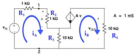
(a) What is the voltage  $v_{\text{OUT}}$  when the input voltage,  $v_{\text{IN}}$  is 2 Volts?
