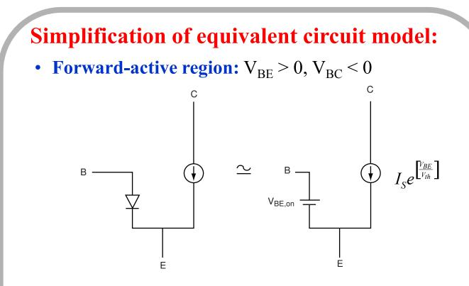
For today's technology:  $V_{BE,on} \approx 0.7 \ V. \ I_B$  depends on outside circuit.
