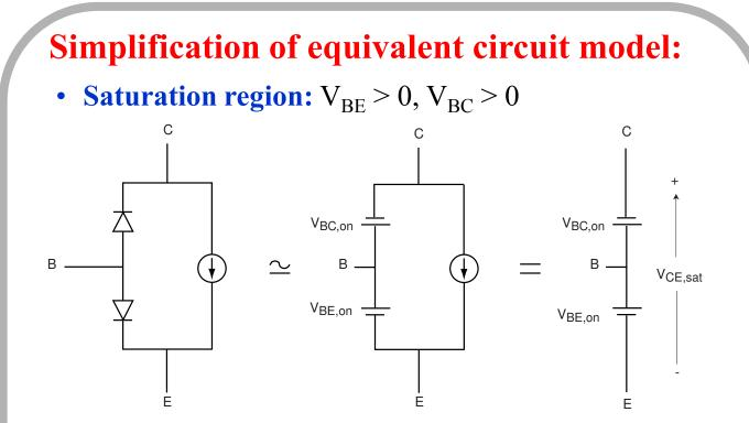
For today's technology:  $V_{CE,sat} \approx 0.1~V.~I_C$  and  $I_B$  depend on outside circuit.
