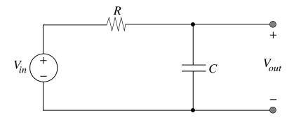
• Replacing the capacitor by its impedance,  $1/(j\omega C)$ , we can solve for the ratio of the phasors  $V_{out}/V_{in}$
