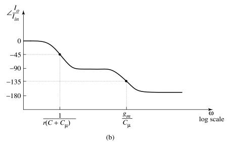
• Frequency at which current gain is reduced to 0 dB is defined at  $f_{T}$ :
