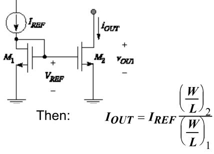
I<sub>OUT</sub> scales with I<sub>REF</sub> by W/L ratios of two MOSFETs ⇒ *Current Mirror Circuit*
