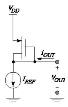
Same operation and characteristics as NMOS voltage source. PMOS needs to be larger to attain the same  $R_{\text{out}}$ .
