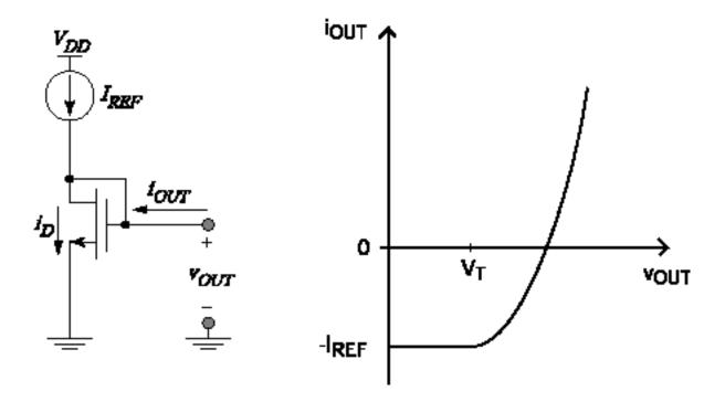
$V_{GS} = V_{DS}$  takes a value needed to sink current
