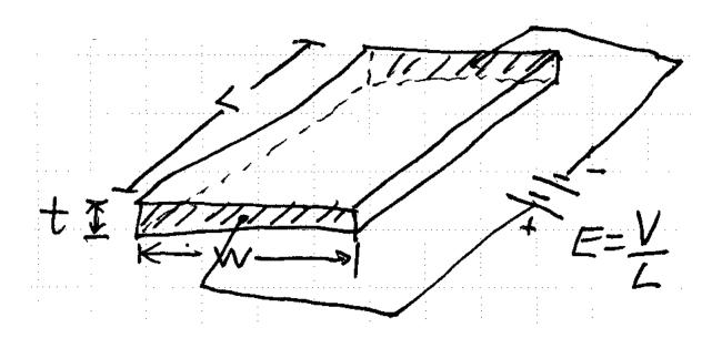
Area: w x t n-type slab of Si Fabricated by ion implantation from top As long as doping is uniform along L, no diffusion along L Therefore, only drift current along L Note: doping need not be uniform along t (as you will see)
